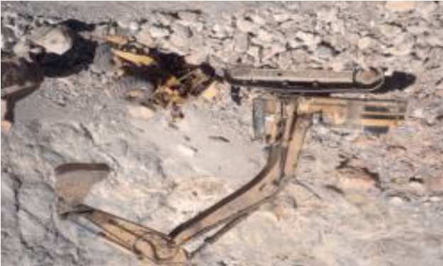
Figure 2: Work machine fell from a height of 70 meters in a quarry in Akçığek.
